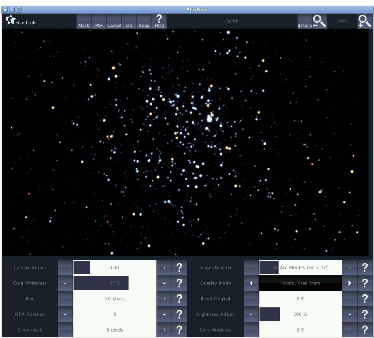
Illustration 27 - The Synth module interface with an image of M11 (image acquisition by Jim Misti).
