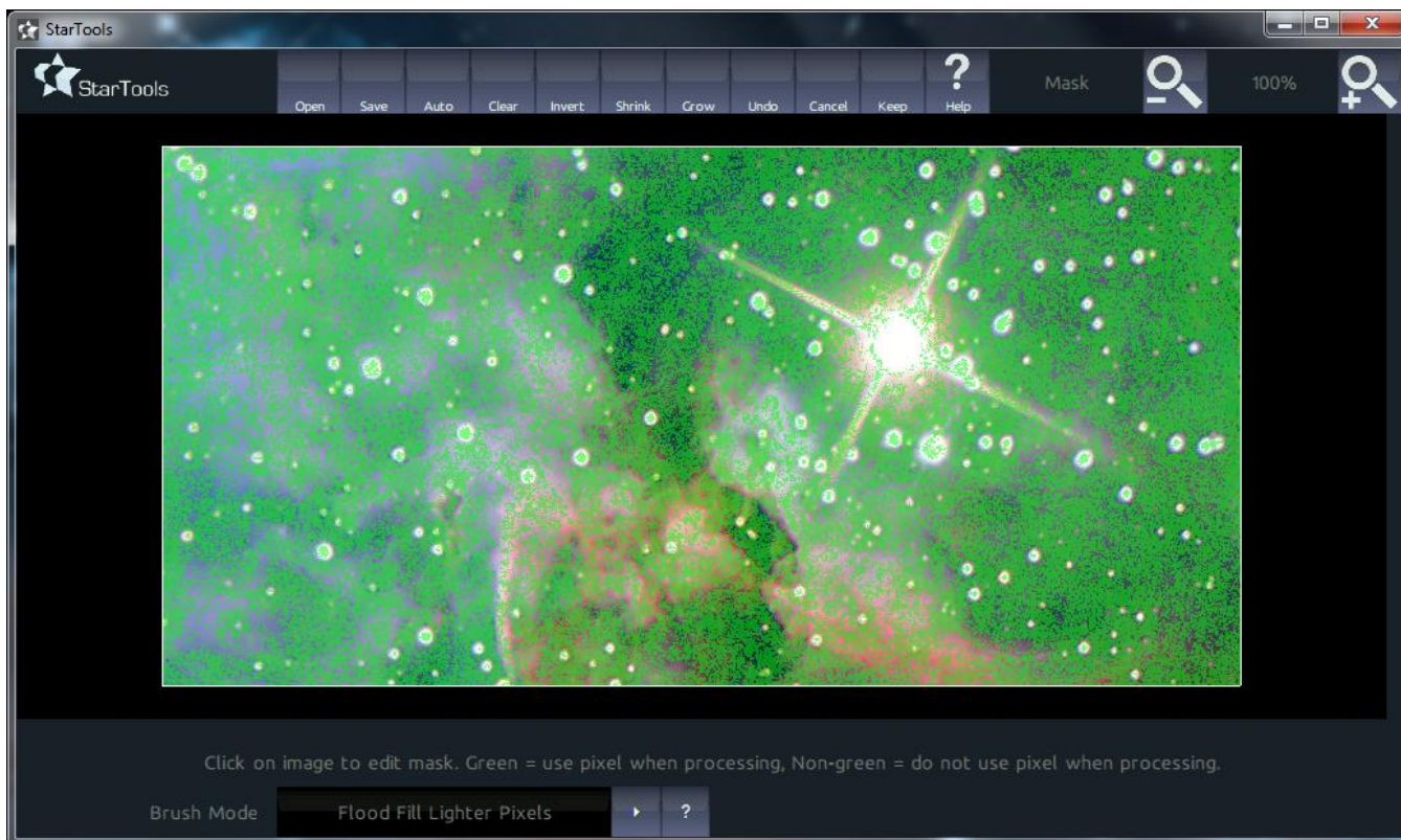
Illustration 79 - The newly generated mask with 'noisy' pixels tagged.
